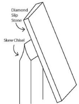
Then place the stone on the long flat edge behind the long point of the skew.
