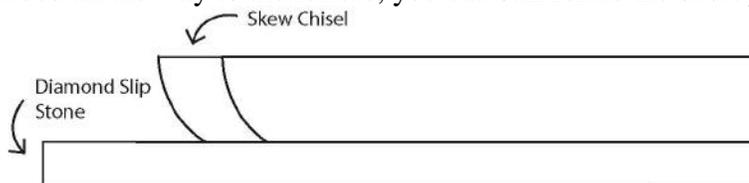
Honing is excellent following grinding to refine the edges, but also is used to keep the edges sharp while working. **Rule:** hone frequently and thereby avoid excessive trips to the grinder.
